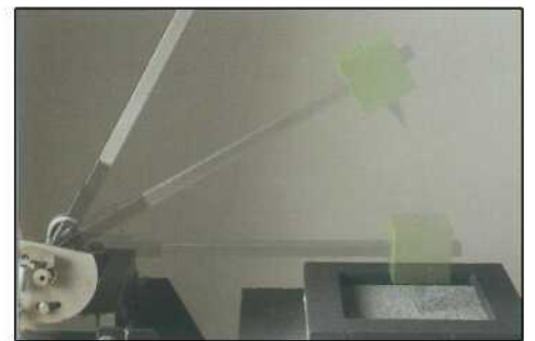
Test for resistance to dynamic indentation.
