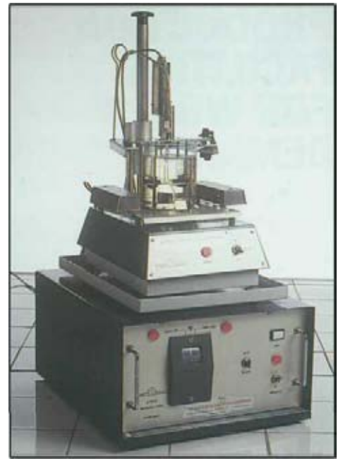
Automatic Ring and Ball test.
