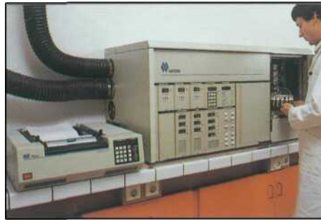
Chromatographic analysis of elastomeric bitumen.
